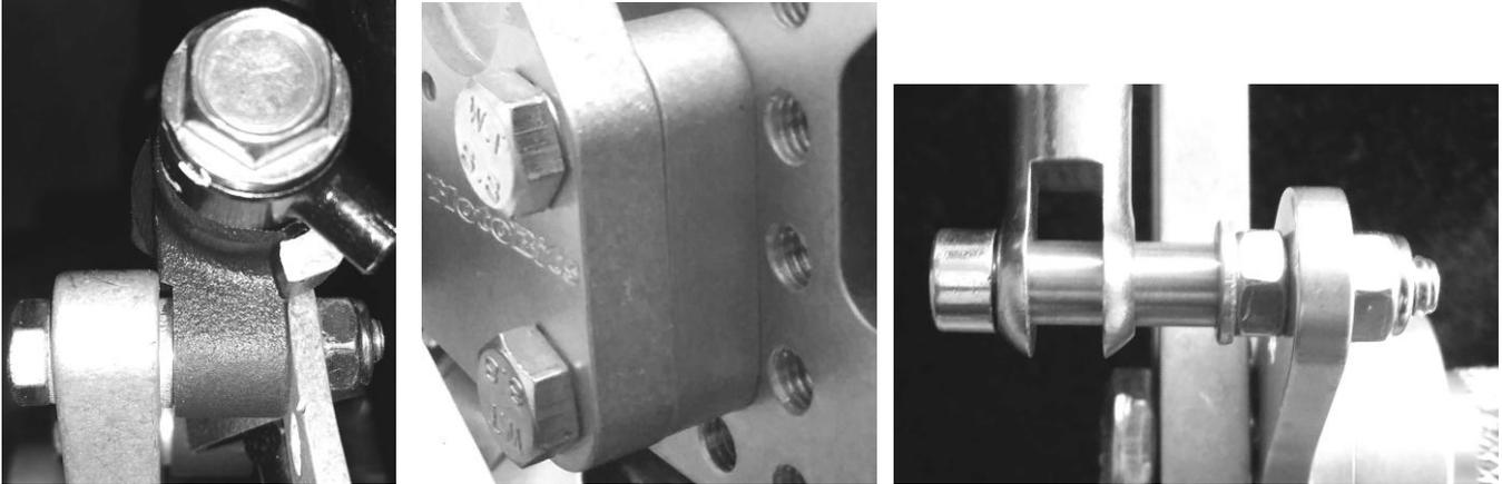
For the Master Cylinder mounting use the 35mm screws with a washer between MC and heelplate. Order is washer-heelplate-washer-MC-locknut. You can also put the strap for the reservoir mounting between the MC and the locknut.
