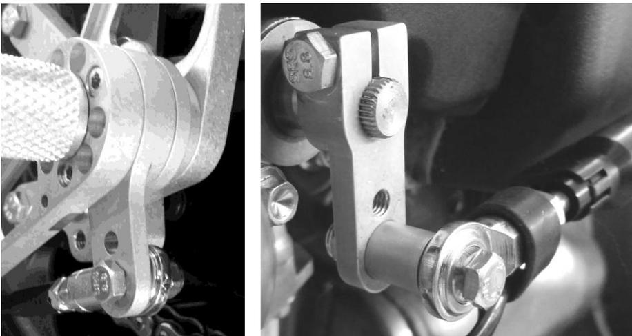
The shift side peg is mounted with a slightly longer screw (number 8 on diagramme) to accommodate the two spacers between the heelplate and the peg. The smaller spacer goes against the heelplate, with the larger against the peg and lever. The photos show positions for standard shift.
