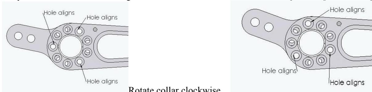
Three equally-distant holes will always align. Use the provided socket-head capscrews and lock washers in the three aligned holes.
