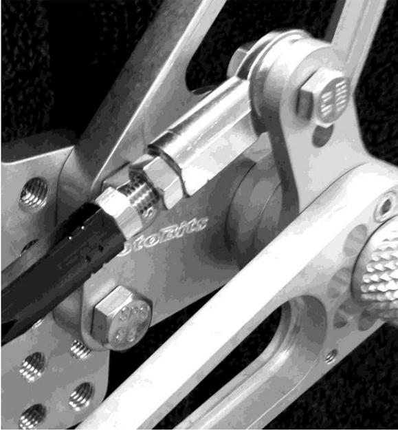
Rotate the collar on the shift lever to point upward instead of downward. This reverses the lever movement but does not change the forces seen by the quickshifter sensor and transmission. No reflashing of the ECU is needed.
