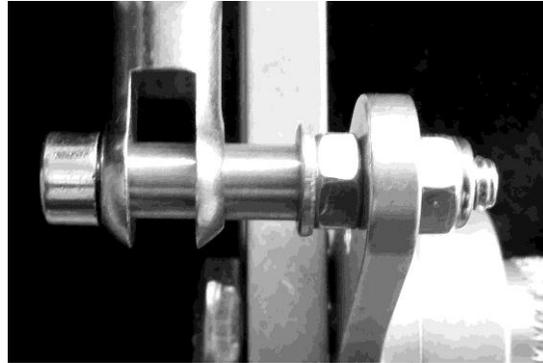
Brake MC is funky. Need 35mm screws, with a washer between MC and heelplate. Goes washer-plate-washer-MC-locknut
