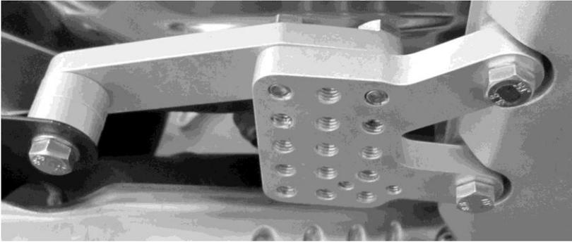
Going to GP shift on models with quickshifter, you will need to rotate the collar on the lever rather than flipping over the shift-shaft arm. This avoids confusing the switch between push/pull.
