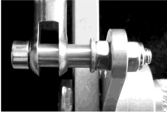
Brake MC is mounted inboard of the heelplate. Use the 35mm screws, with a washers. Goes washer-plate-MC-locknut
