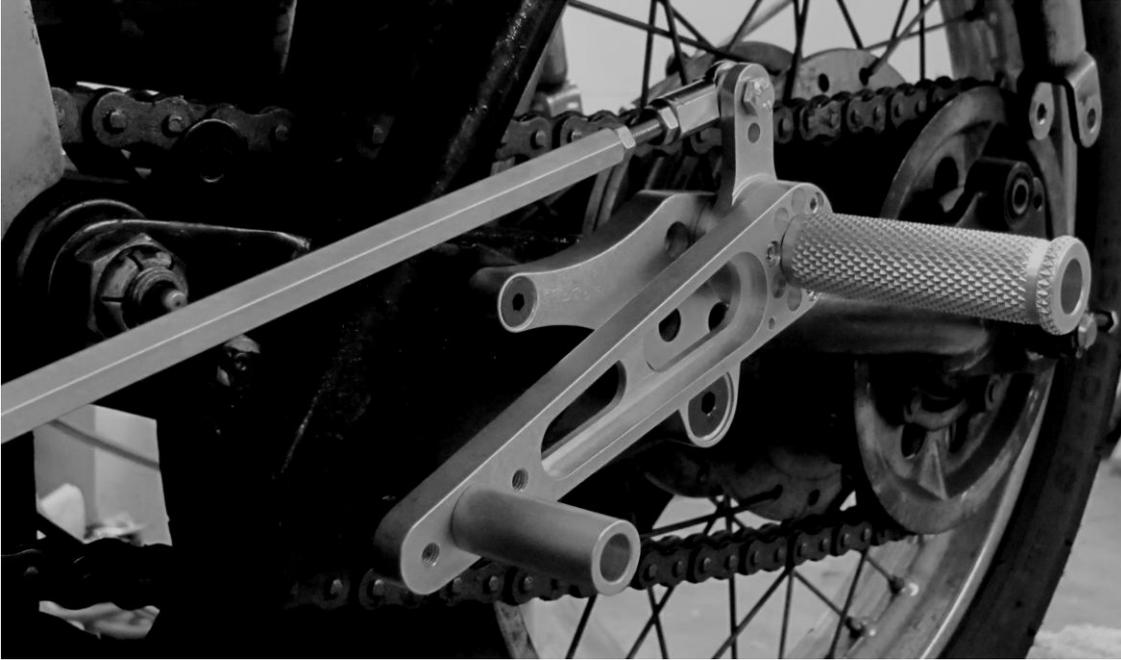
1. Remove the stock footpeg assemblies, including passenger pegs. The rearsets mount in the location of the passenger pegs.
