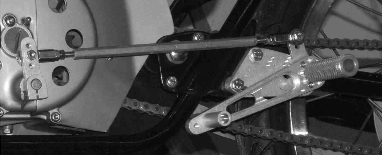
1. Remove the stock footpeg assemblies, including passenger pegs. The rearsets mount in the location of the passenger pegs.
