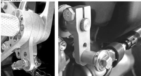
The shift side peg is mounted with a slightly longer screw (number 8 on diagramme) to accommodate the two spacers between the heelplate and the peg. The smaller spacer goes against the heelplate, with the larger against the peg and lever. The photos show positions for standard shift.
