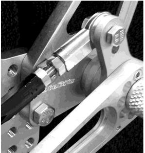
Rotate the collar on the shift lever to point upward instead of downward. This reverses the lever movement but does not change the forces seen by the quickshifter sensor and transmission. No reflashing of the ECU is needed.
