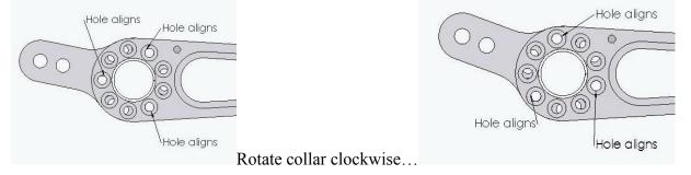
Three equally-distant holes will always align. Use the provided capscrews in the three aligned holes.
